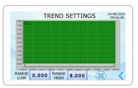
**Graph Settings**: Set high and low limits to visualize real-time channel data and behaviour through a live graph.
